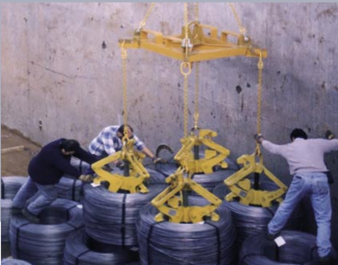
Wire coil inner tong in 4-times combination with adapter crosshead
