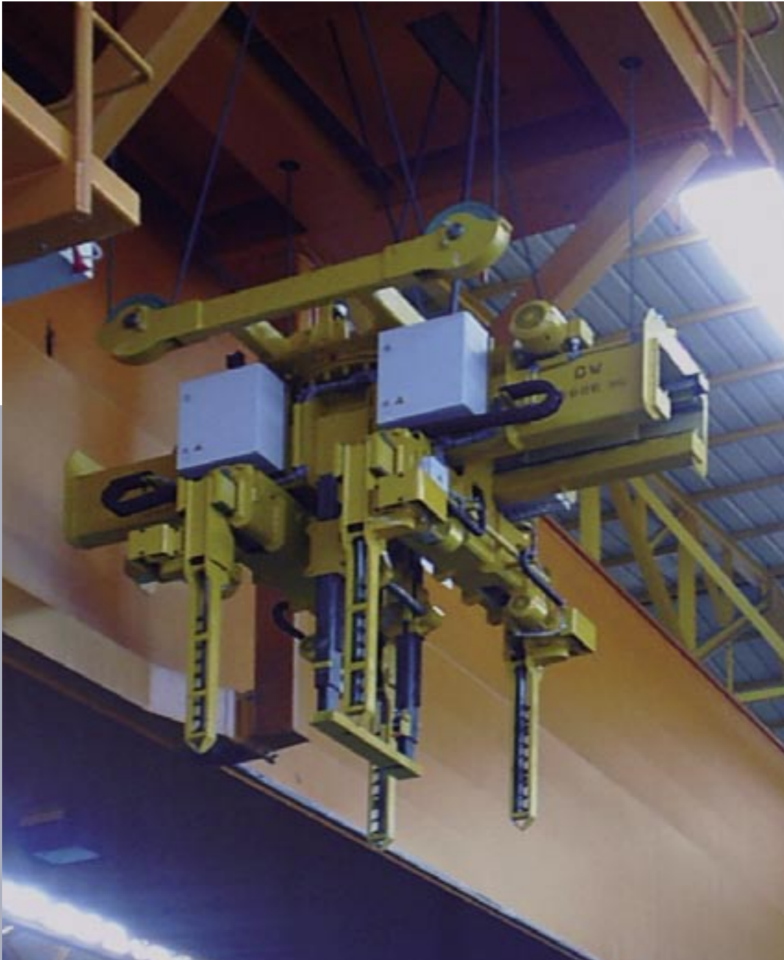
Electrohydraulic structural steel mesh grab, internal grab, with slewing gear and pulley attachment, grab width adjustable by length and cross, mobile feet, with electronic internal height adjustment for different mesh lifting heights
