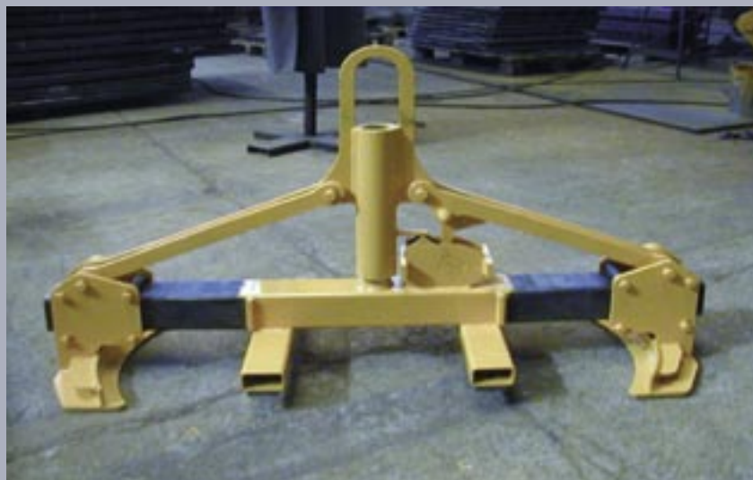
Coil tongs for vertical transport, each with load capacity of up to 5 t
