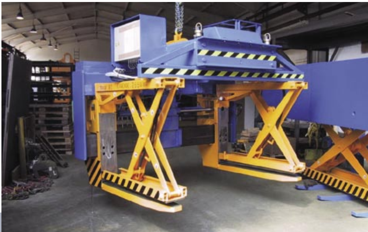
Electrohydraulic board lifts with hold-down function and grab width adjustment
