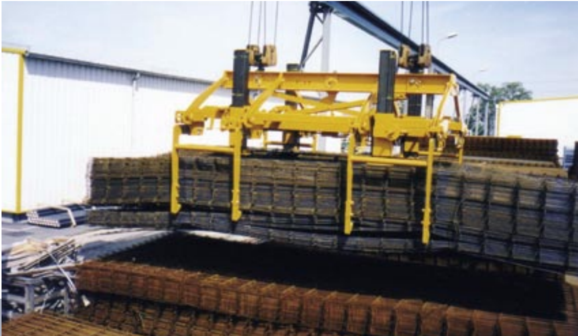
Simple mechanical structural steel mesh grab with automatic step-by-step motion and manual table height adjustment using crank handle
