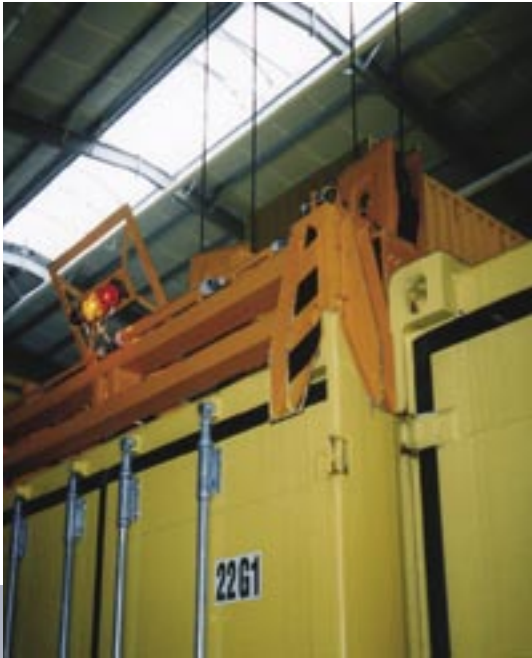
Electrohydraulic container spreaders for 20' ISO containers and interchangeable bodies
