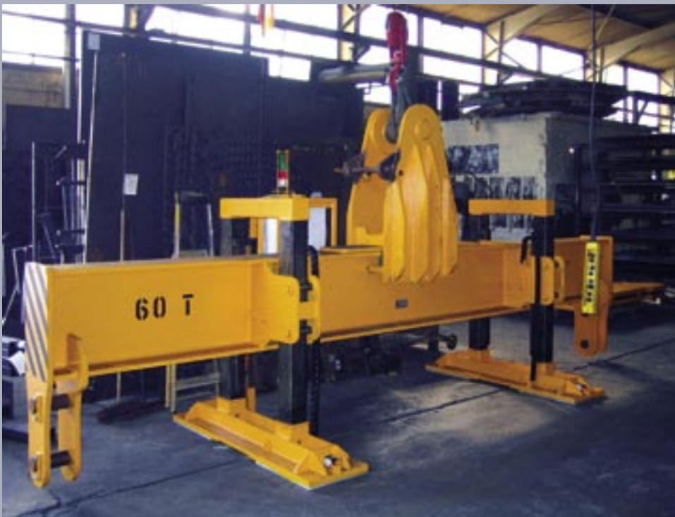
Electromotive doubling drum transport crossheads with mobile grab pins for the construction units
