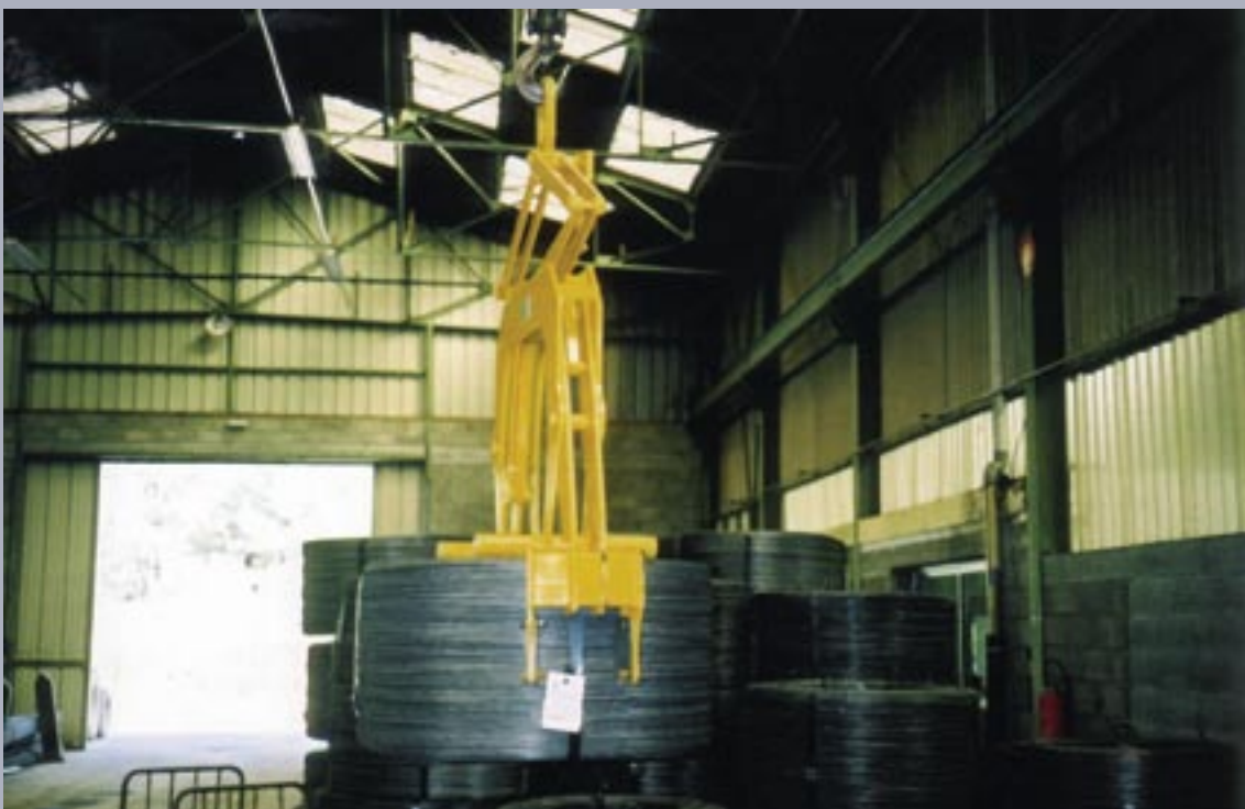
Wire coil inner tongs in very narrow special construction, also with large internal height
