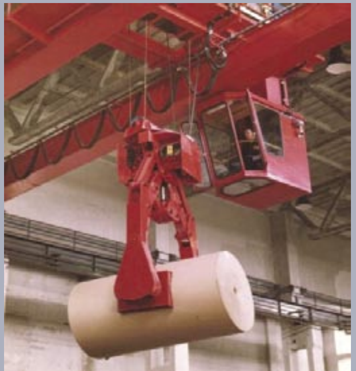
Electrohydraulic paper roll grabs with 90 degree slewing gear Mechanical long hook crosshead
