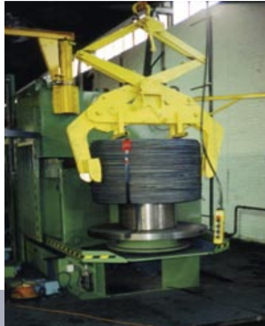
Wire coil outer tongs, small design, suitable for laying coils on bobbin winders.
