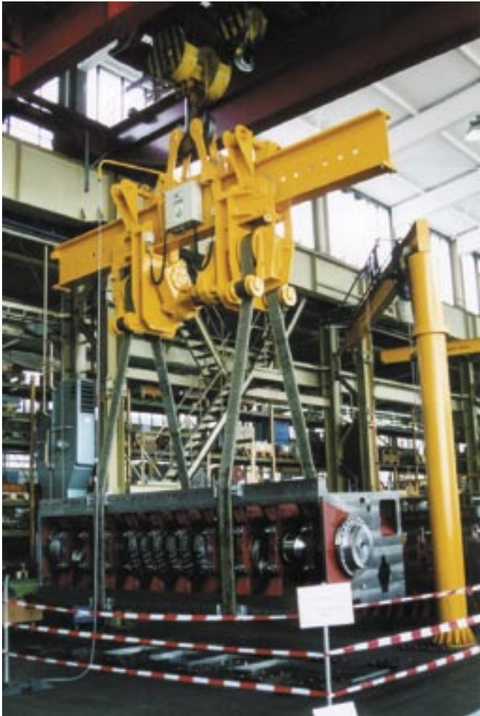
Electromotive turning crosshead with grid adjustment
