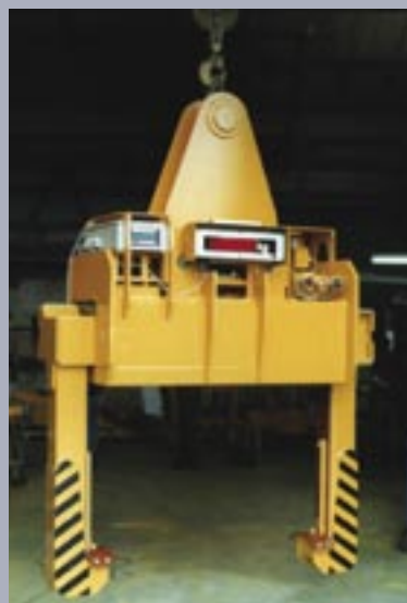
Telescopic coil grabs with integrated weighing mechanism
