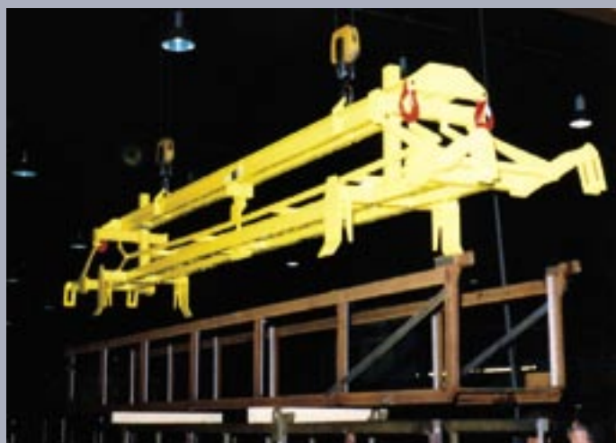
Cradle grabs with manual stacking machine for frontal lifting of stackable cradles
