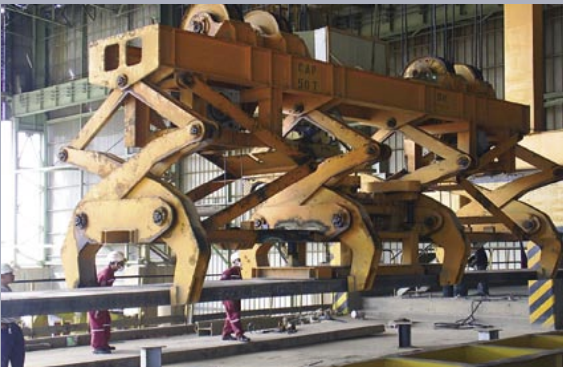
Electromotive four-times slab tongs with electric lifting mechanism and electric table height adjustment
