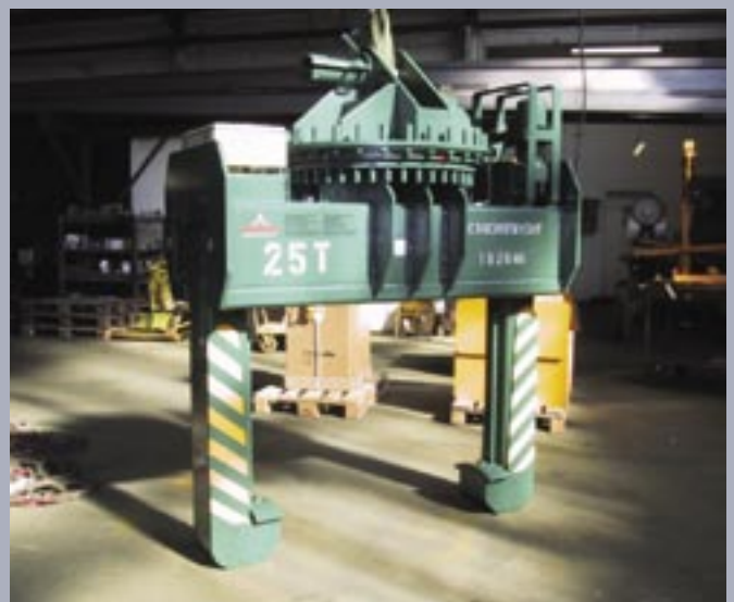
Telescopic coil grabs with slewing gear
