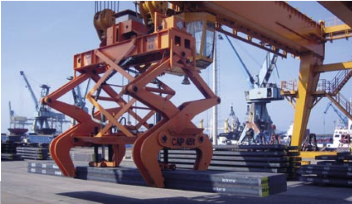
Electrohydraulic slab tongs with electronic lifting mechanism and hydraulic table height adjustment, but with two-point attachment
