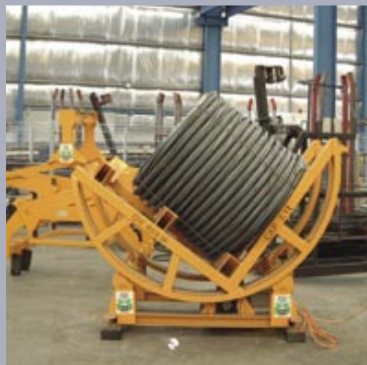
Electromotive tilting table for turning coils up to 90°
