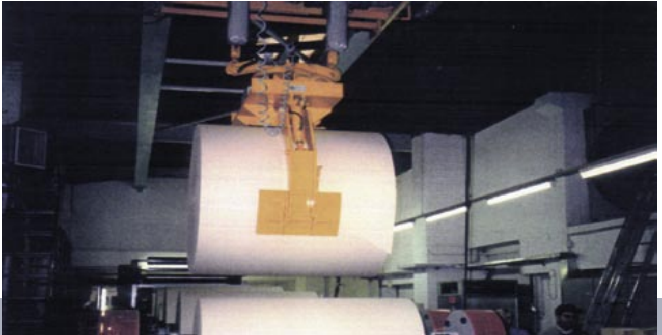
Electrohydraulic paper roll tongs with slewing gear
