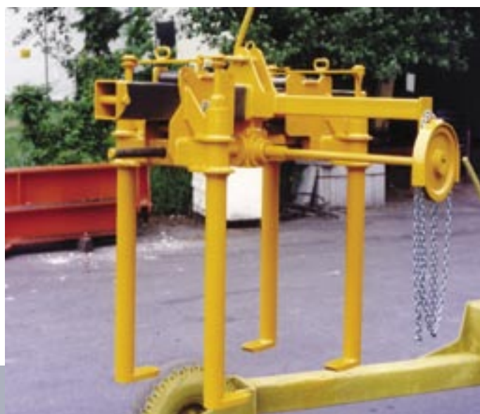
Spindle grabs for sheet boards with mobile grab feet
