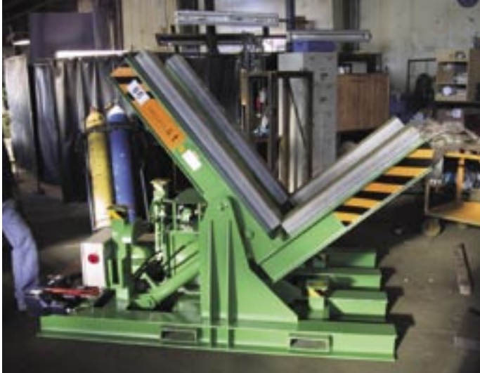
Electrohydraulic tilting tables to tip coils by 90° up to a load capacity of 40 t
