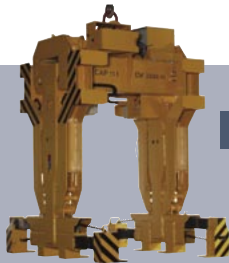
Electromotive telescopic sheet stack grabs with fixed central grab feet, with additional, manually removable grab feet and electrohydraulically retractable outer grab feet
