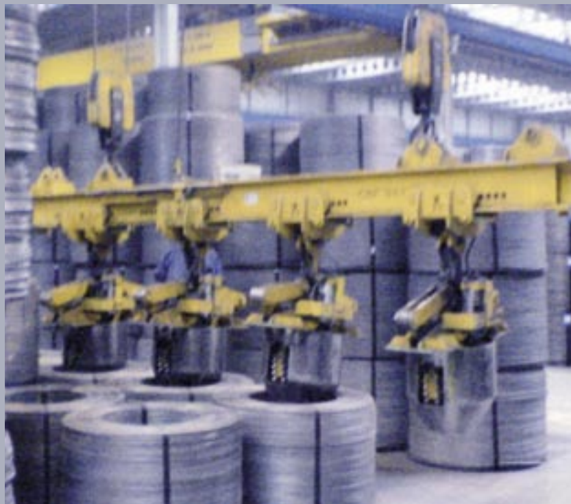
Special crosshead with 4-times arrangement of wire coil inner tongs and electromagnetic release device. Grab width can be adjusted individually by hand using roller chassis and locking pin.
