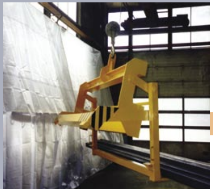
Stand control device with automatically movable counterweight
