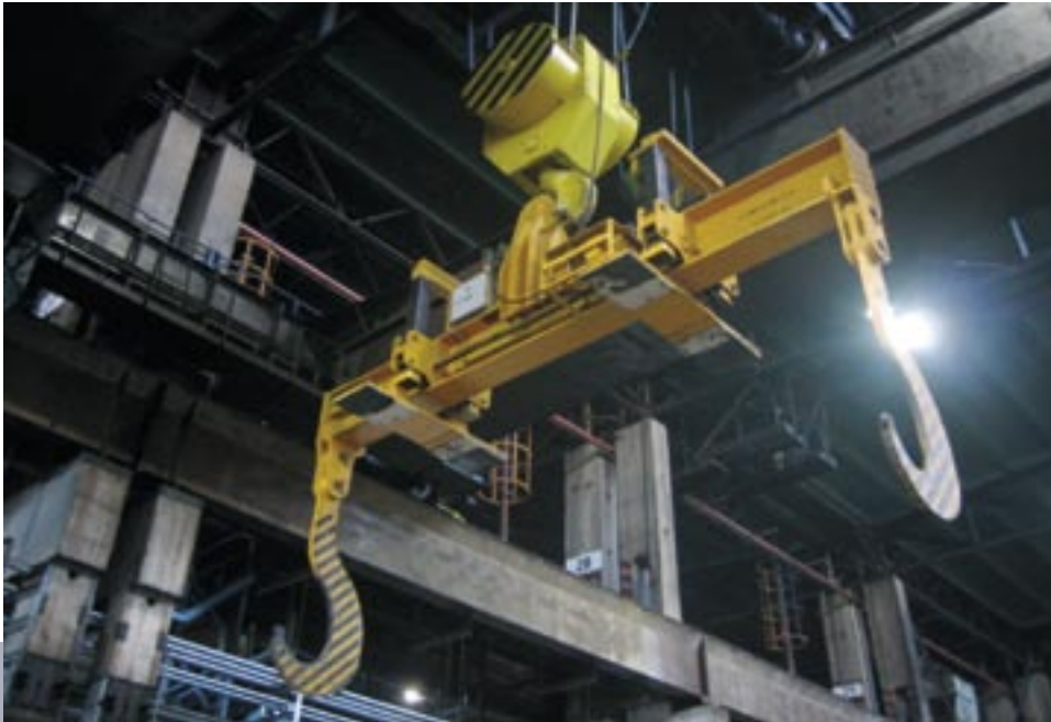
Electromotive doubling drum transport crossheads for grabbing doubling drums with construction units
