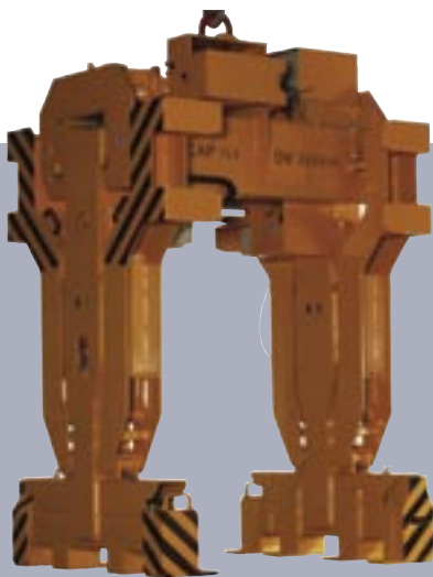
Electromotive telescopic sheet stack grabs with fixed central grab feet, with additional, manually removable grab feet and electrohydraulically retractable outer grab feet
