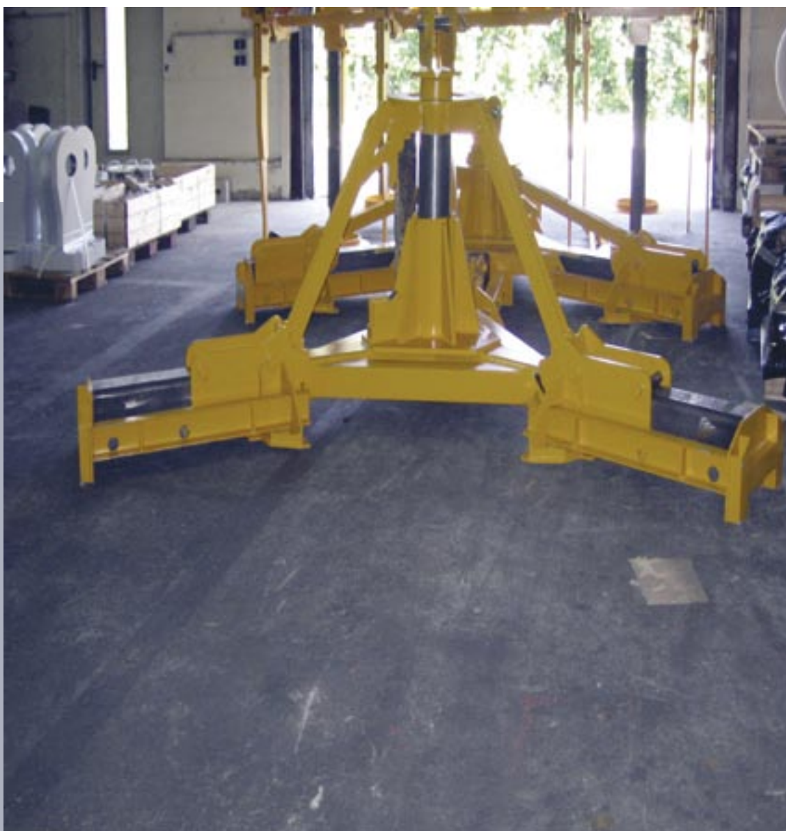
Mechanical convector sheet tongs to grab convector sheets in annealing plants.
