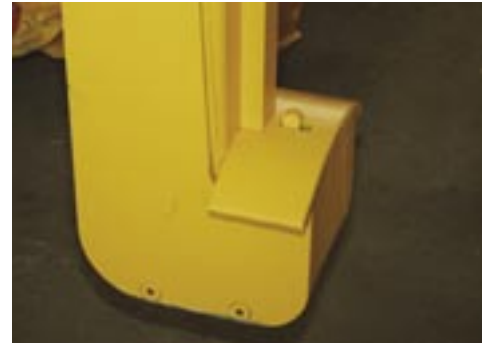
Feet contact banks to prevent unauthorised opening when loaded
