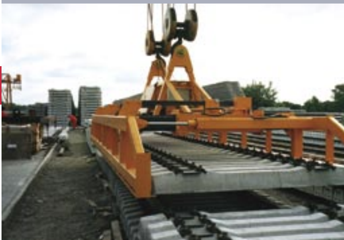
Concrete sleeper grab for 30 sleepers of different lengths
