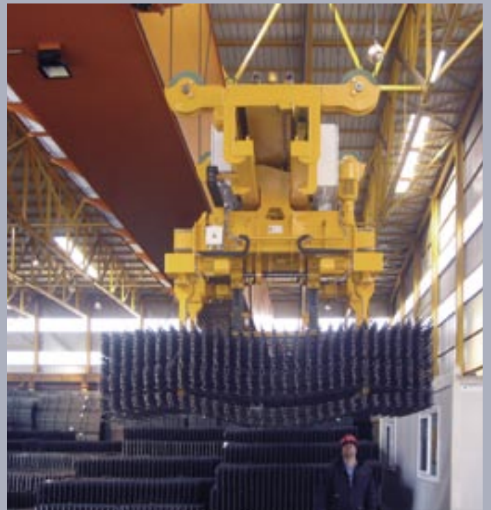
Electrohydraulic structural steel mesh grab, internal grab, with slewing gear and pulley attachment, grab width adjustable by length and cross, mobile feet, with electronic internal height adjustment for different mesh lifting heights
