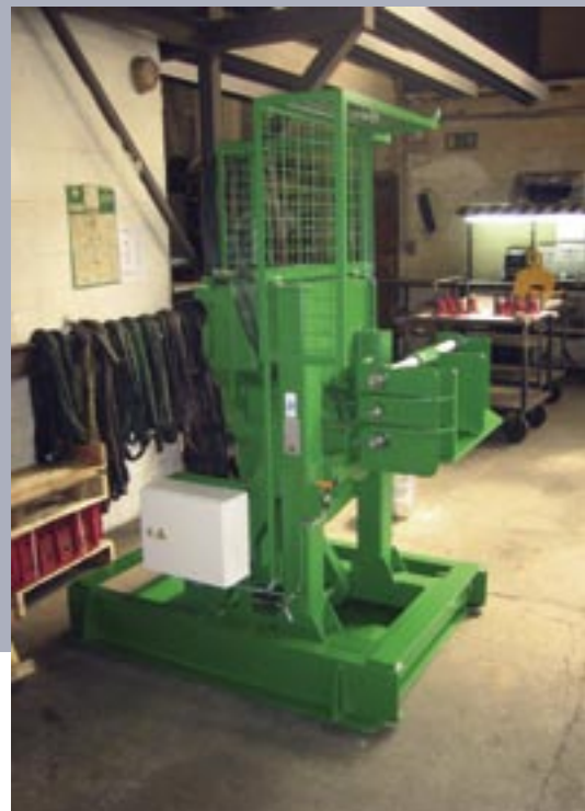
Electromotive beam turning equipment for rolled steel sections
