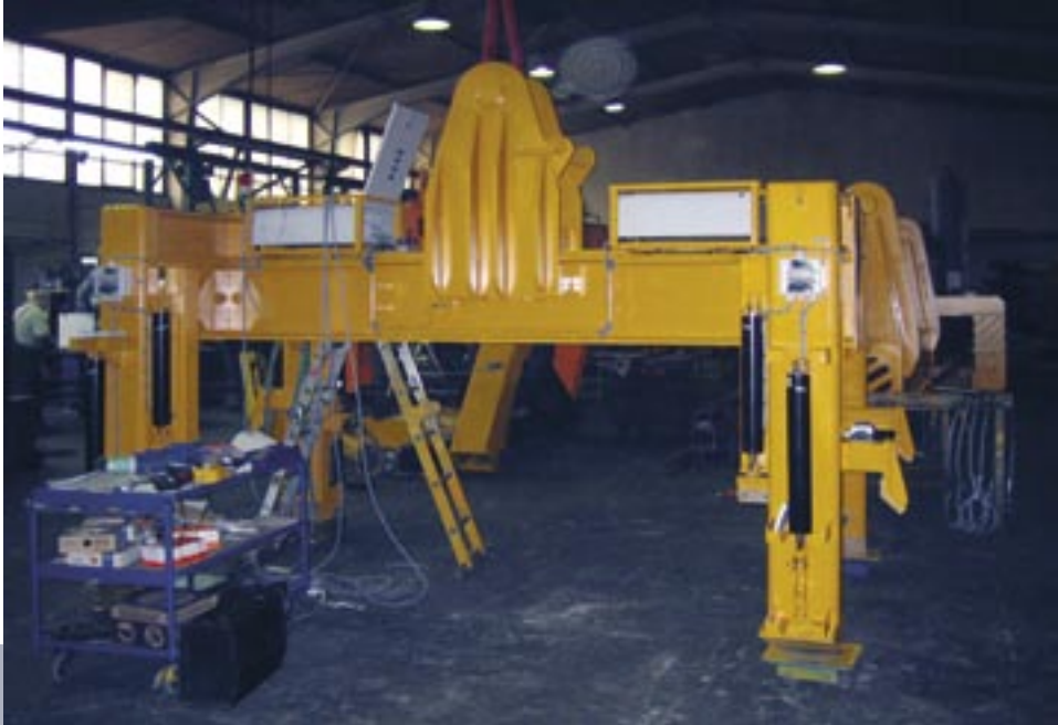
Electromotive doubling drum transport crossheads with mobile grab pins for the construction units
