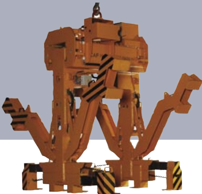
Electromotive telescopic sheet stack grabs with fixed central grab feet, with additional, manually removable grab feet and electrohydraulically retractable outer grab feet
