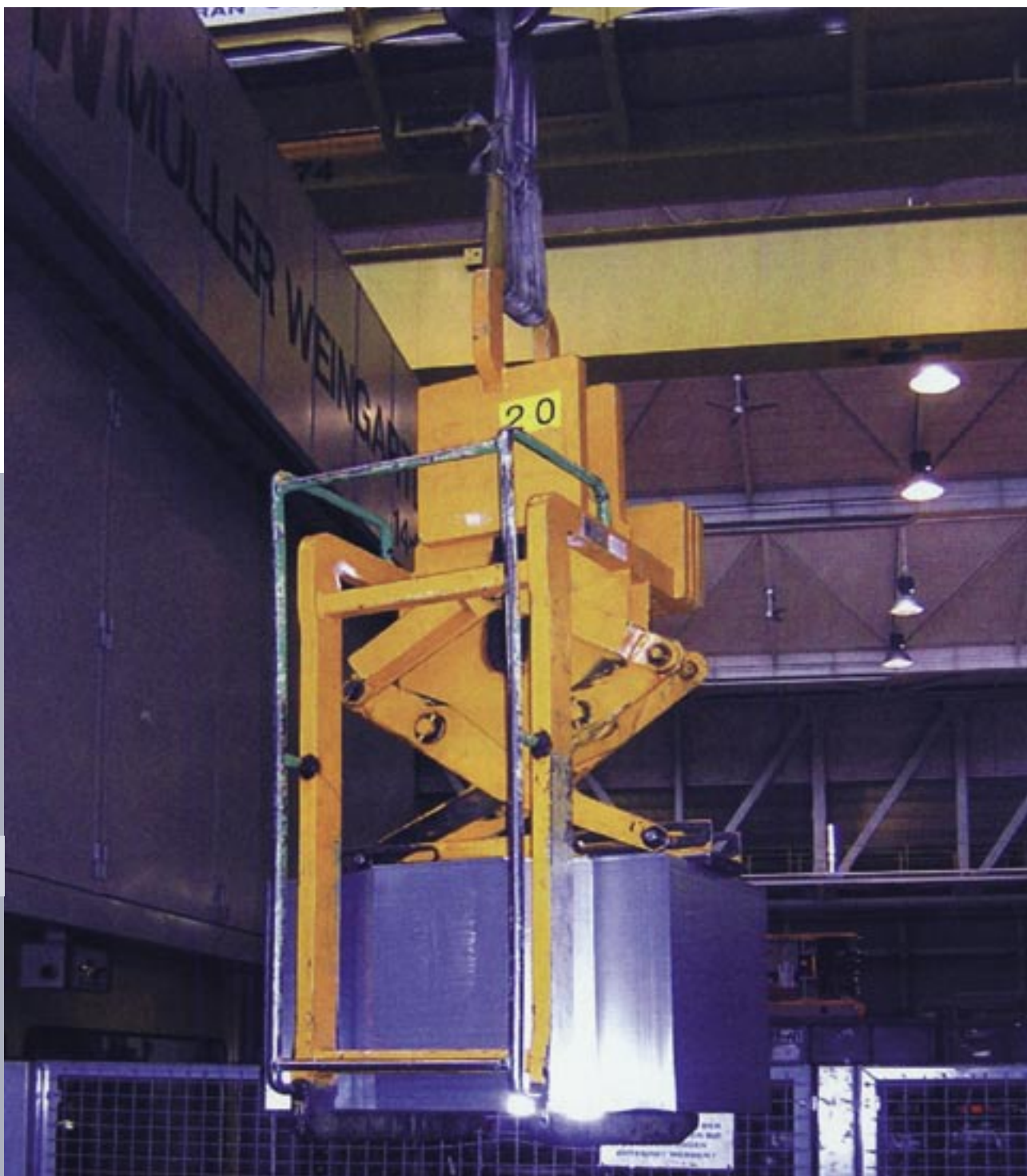
Board lifts with mechanical hold-down function
