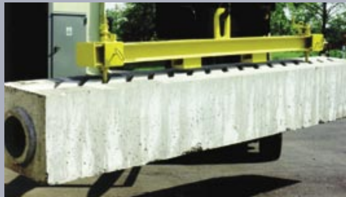
Special crossheads with concrete lifting pins
