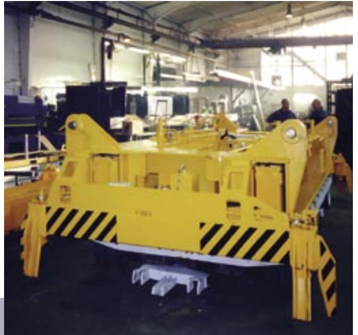
Container spreaders electrohydraulically telescopic from 20' to 40'
