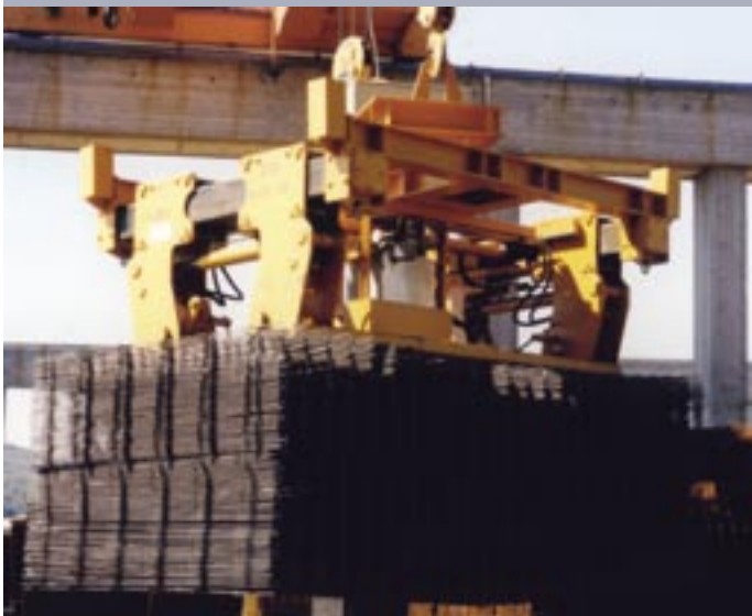
Electrohydraulic structural steel mesh grab, internal grab, with horizontal slewing gear with feet adjustable by length and cross for the different mesh types
