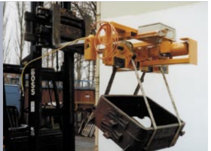
Turning crosshead as ancillary equipment - direct current supplied to the starter battery
