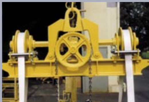
Turning crosshead with worm gear pair drive
