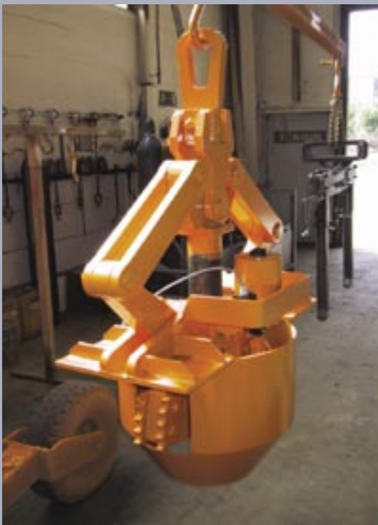
Wire coil inner tongs with electromagnetic opening and closing device and leading-in funnel
